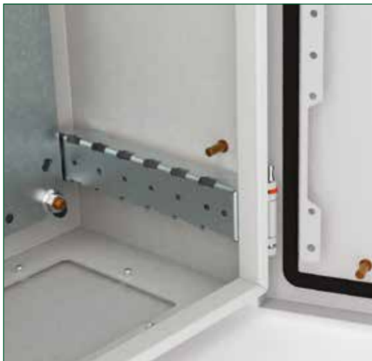
Wiring support, creation of an internal structure and depth adjustment of the accessories at 25 mm intervals thanks to the universal cross-pieces (with front fastening to the universal brackets).
